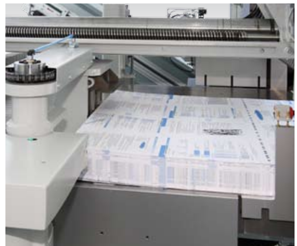
Automatic turning of the layer on the rear-table; up to 4 cuts are possible without any operator's intervention
